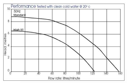
NOTE: These magnetically coupled pumps are designed for use with clean fluids.
